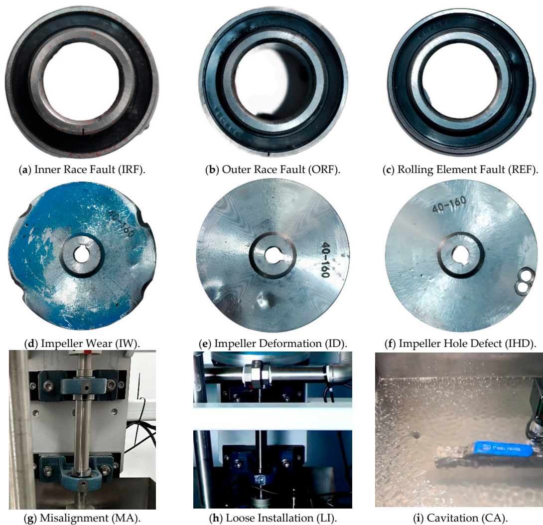
Figure 7. Schematic diagram of simulated fault types in the submersible centrifugal pump.
