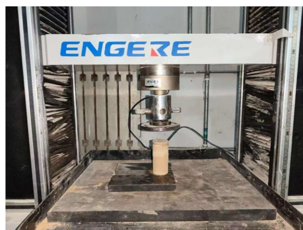
Figure 7. Unconfined compressive strength (UCS) testing apparatus and setup.
