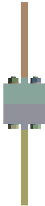
Figure 1. Overall configuration of the T-flange joint specimen used in the finite element analysis.
