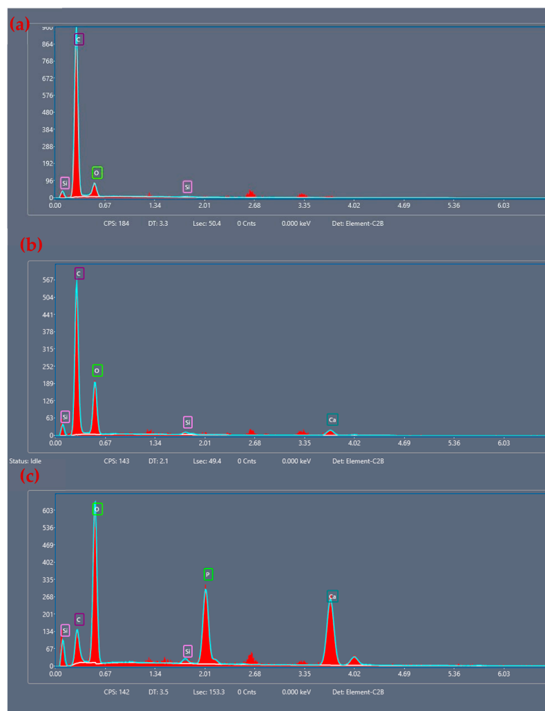
Figure 2. Energy dispersive X-ray spectroscopy spectrum of (a) unactivated water hyacinth biochar (WHB), (b) eggshell-treated activated water hyacinth biochar (EP-WH), and (c) double activated water hyacinth biochar (EP-WH-PA).
