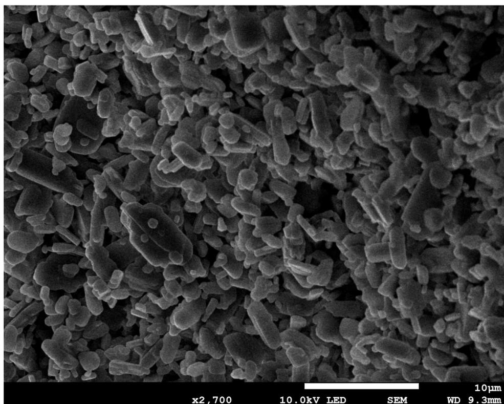
**Figure 4.** SEM picture of raw CEL powder.
