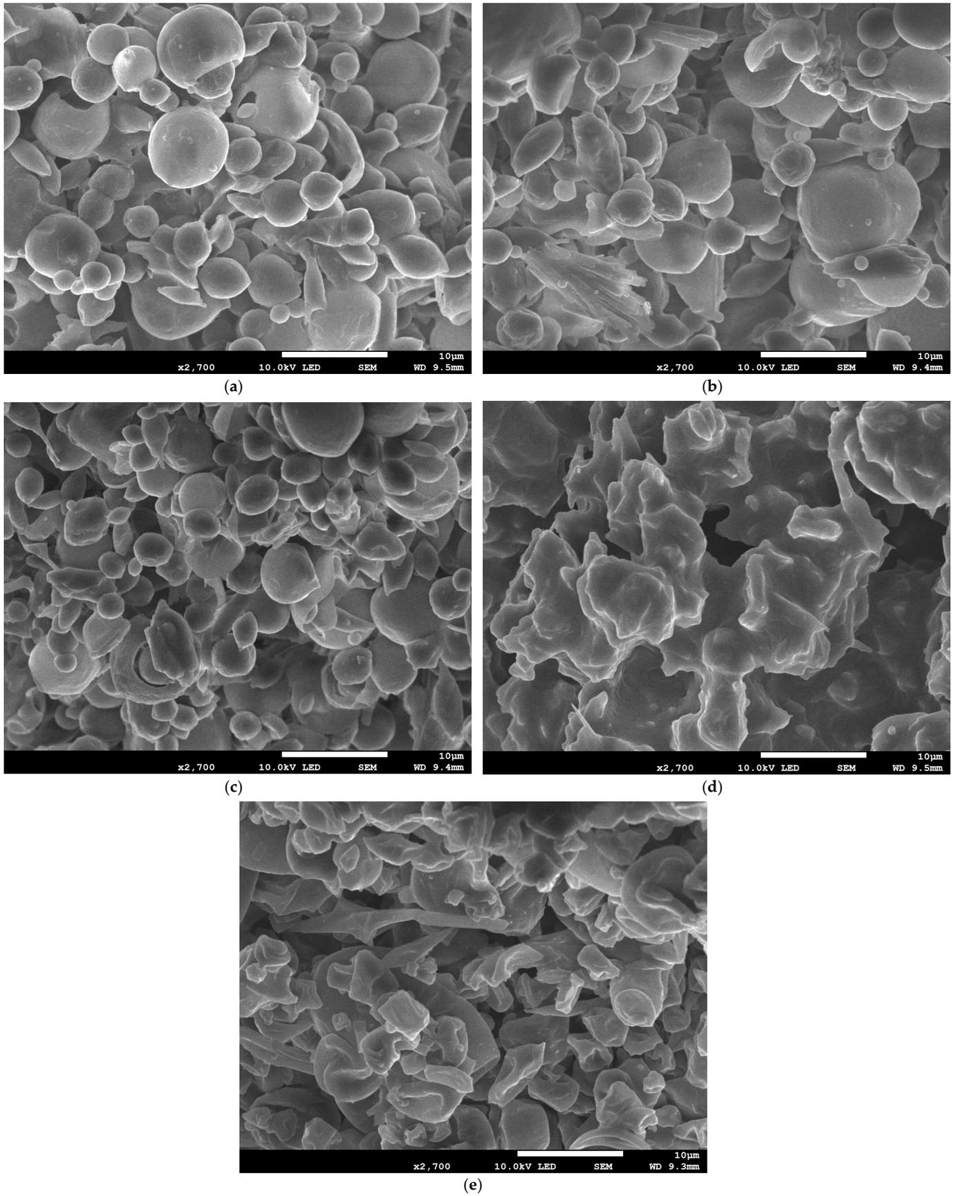
**Figure 5.** SEM picture of (a) freeze-dried formulation 1; (b) freeze-dried formulation 2; (c) freeze-dried formulation 3; (d) freeze-dried formulation 4; (e) freeze-dried formulation 5.
