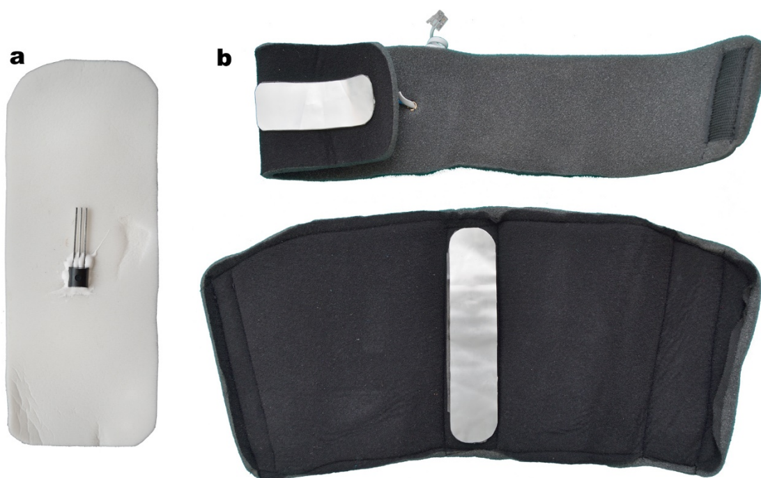
Figure 4. (a) Thermic sensor attached to the metallic foil. (b) Thermic sensors for the distal and proximal component.
