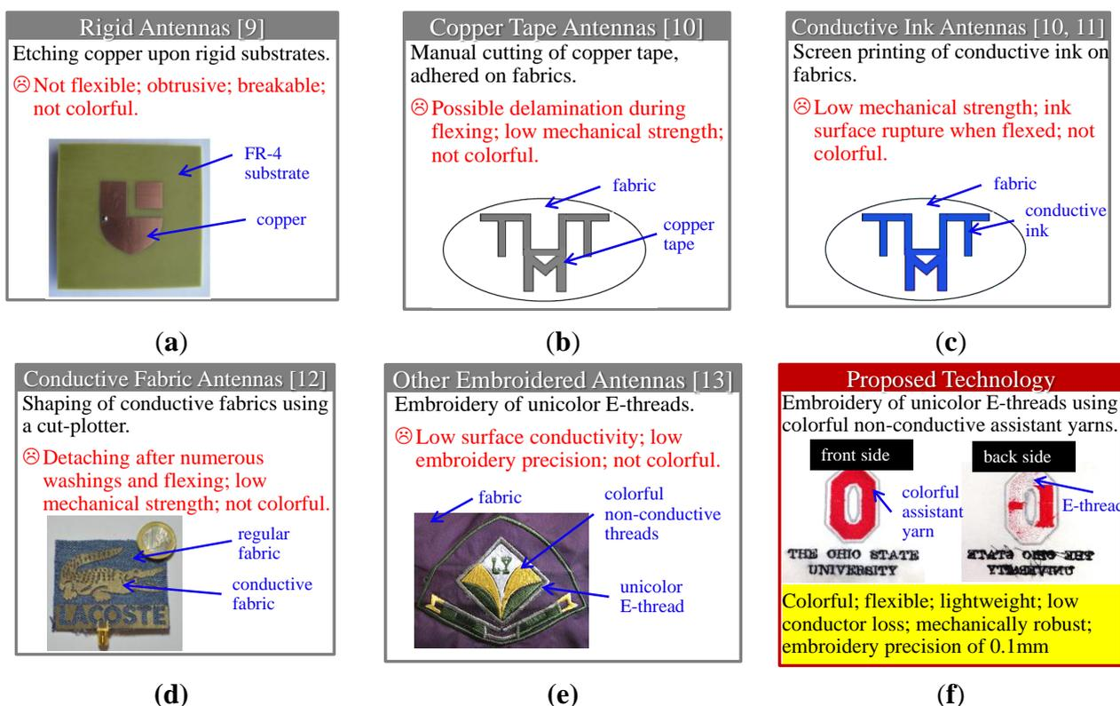
**Figure 1.** Former technologies used to realize wearable logo-shaped antennas: (a) rigid antennas © John Wiley and Sons [9]; (b) copper tape antennas [10]; (c) conductive ink antennas [10,11]; (d) conductive fabric antennas © IEEE [12]; (e) other embroidered antenna © IEEE [13]; versus (f) proposed technology.
