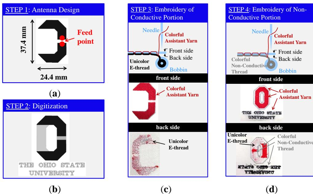
**Figure 2.** Proposed technology for colorful logo antennas: (a) STEP 1: antenna design; (b) STEP 2: digitization; (c) STEP 3: embroidery of conductive parts; (d) STEP 4: embroidery of non-conductive parts.
