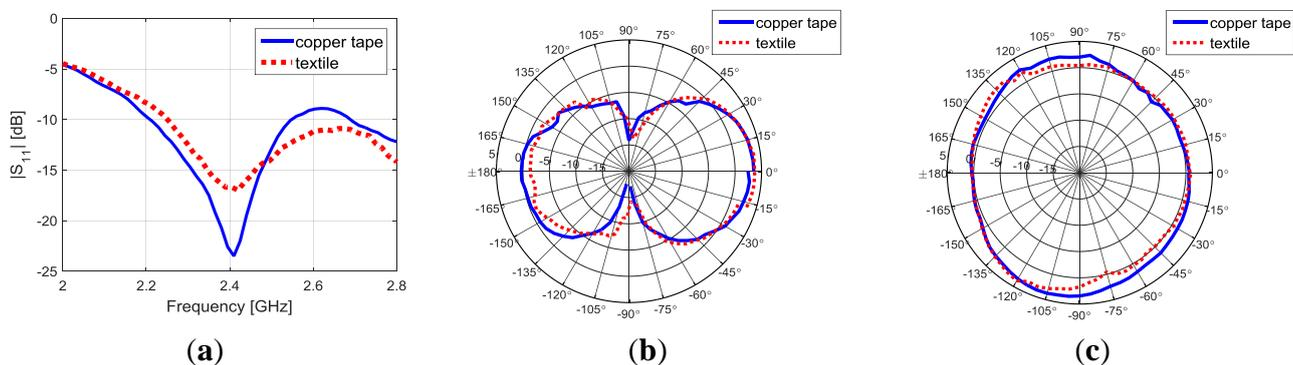
**Figure 4.** Measured performance of the textile and copper tape dipole prototypes: (a) reflection coefficient,  $|S_{11}|$ ; (b) E-plane realized gain radiation pattern at 2.4 GHz; (c) H-plane realized gain radiation pattern at 2.4 GHz.
