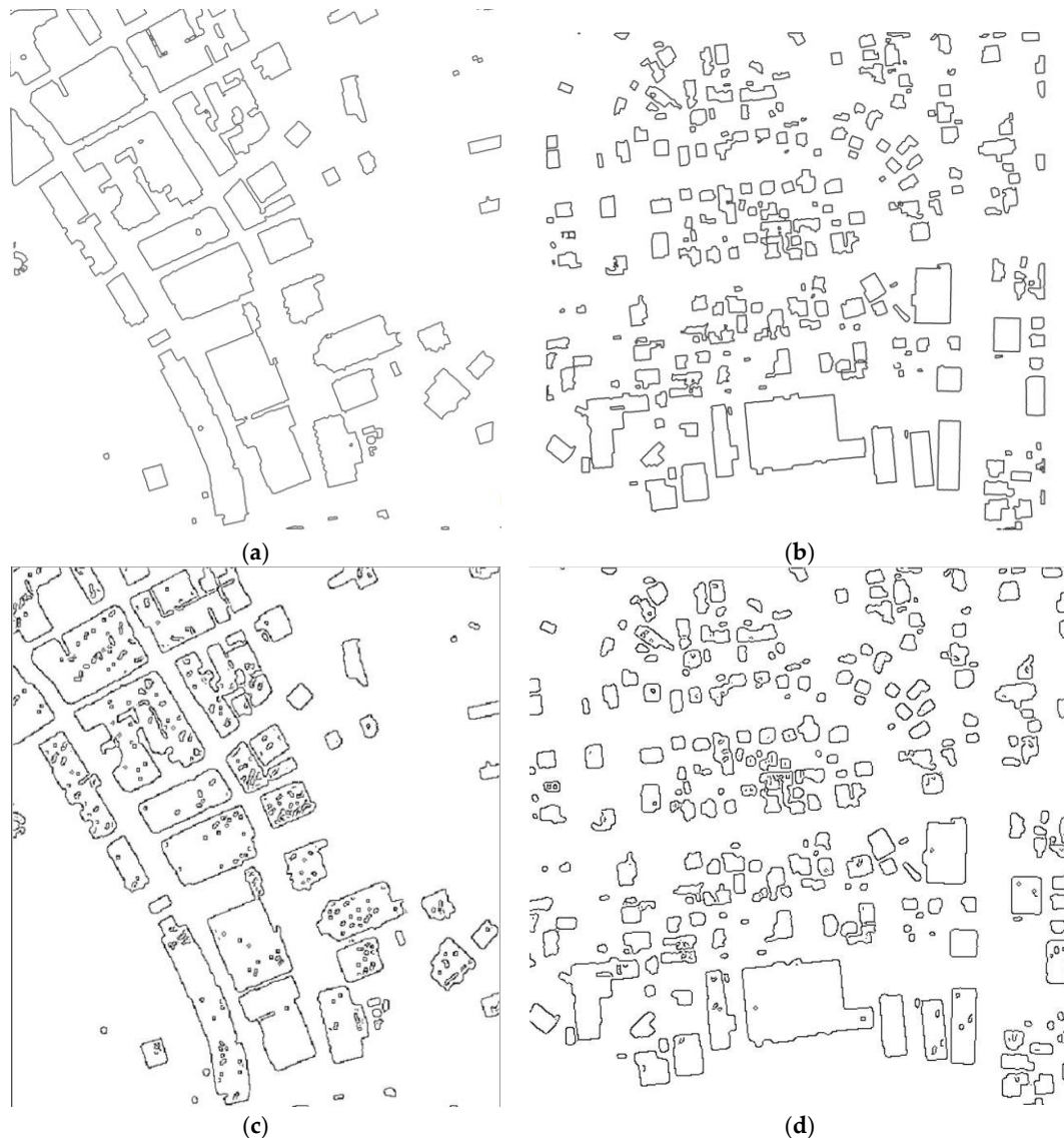
Figure 6. (a–d) Present the result of building outline generation of two regions. Specifically, (a,b) are the result of \alpha -shape algorithm of two regions; and (c,d) are the result of Canny algorithm.
