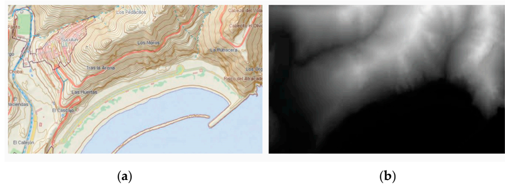
Figure 2. Original contour lines map of Las Teresitas beach (a) and height map (b).
