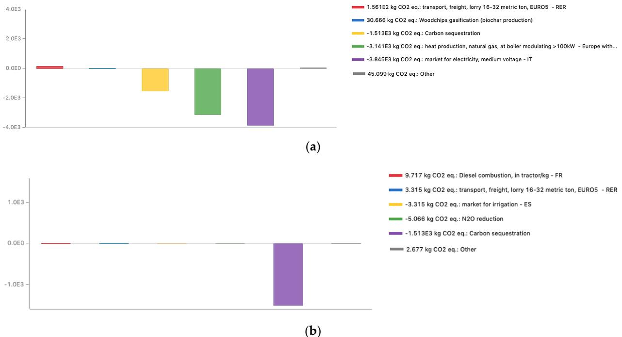
**Figure 4.** Climate change–GWP 100: top 5 contributions impacting category results: (a) Cradle-to-grave analysis; (b) Downstream process.
