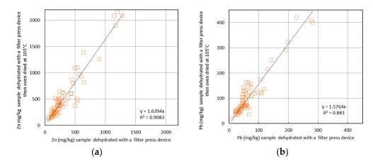
**Figure 10.** pXRF analyses on pressed and part dehydrated samples compared to analyses on samples oven dried at 105  $^{\circ}$ C; (a) Zn and (b) Pb.
