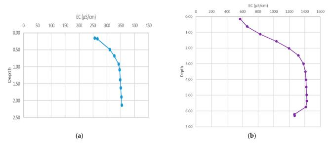
**Figure 9.** Electrical conductivity profile of wells by multiparametric probe ( $\mu$ S/cm): (**a**) BH10 well; (**b**) BH 19 well.
