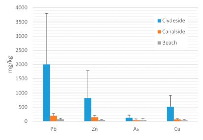
Figure 8. Comparison of mean content in Pb, Zn, As and Cu in the 3 zones.
