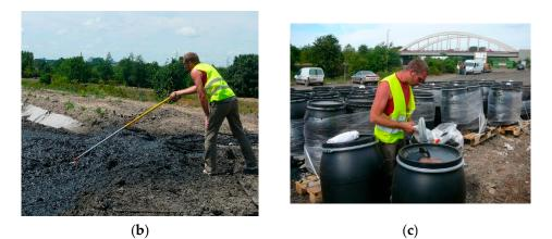
**Figure 1.** Sampling and analysis during sediment loading and unloading: (**a**) Sampling a barge load with a small trowel mounted on a telescopic handle; (**b**) Sampling from an unconsolidated lagoon; (**c**) checking lots before sending to a processing test.
