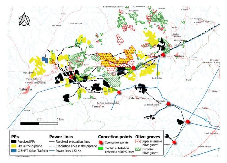
**Figure 1.** PPs and evacuation lines resolved and in the pipeline, connection points, and superintensive and intensive olive groves. La Ribina substation and the power lines (220 kv and 400 kv) that converge at Tabernas substation are not shown for clarity.
