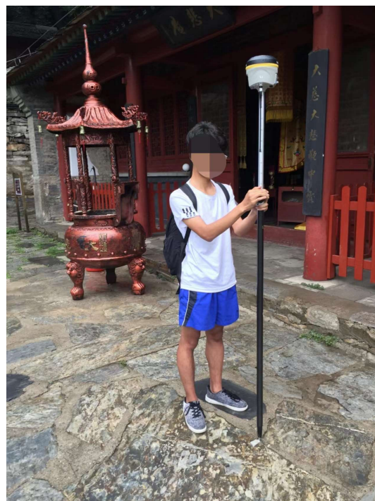
Figure 11. Measuring Point 4 for geographic registration.
