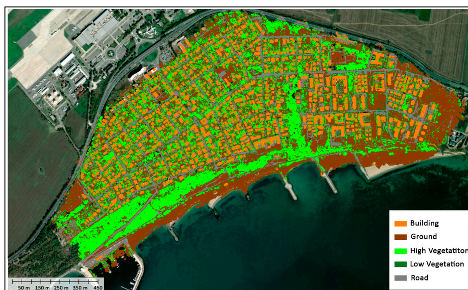
Figure 6. Surface type classification—based on the processed aerial photogrammetry data.
