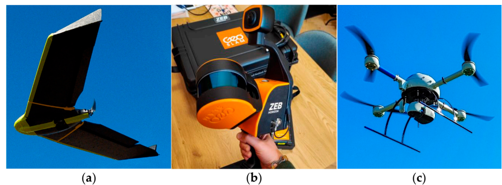
Figure 4. Remote Sensing Equipment: (a) Ag Eagle eBeeX Fixed-Wing UAS; (b) GeoSLAM Zeb Horizon LiDAR; (c) mdLiDAR1000HR Multirotor UAS.
