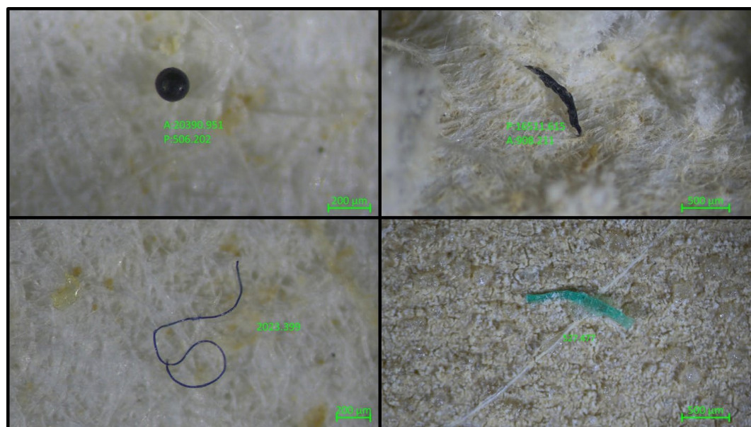
Figure 2. Microplastic particles of diverse morphology and size in sewage sludge-amended pistachio orchard soils.
