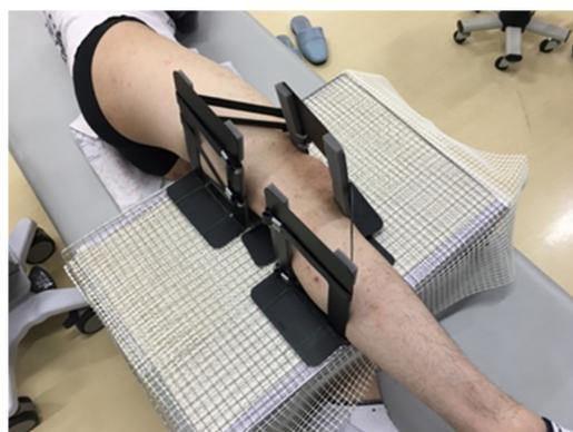
**Figure 1.** Knee Clamping Device. A knee immobilization device was fabricated to hold the knee joint in the extended position. In order to avoid inhibiting the mobility of the deep fascia due to the compression of the lateral part of the lower limb on the test side, one control plate was placed in front of the knee joint, and two control plates were placed distal to the thigh and proximal to the lower leg to immobilize the lower limb.
