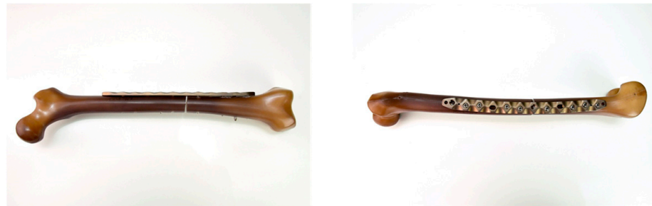
Figure 2. Artificial bone prepared using an osteosynthesis plate (NCB ® femur shaft plate) as an IP reference object.
