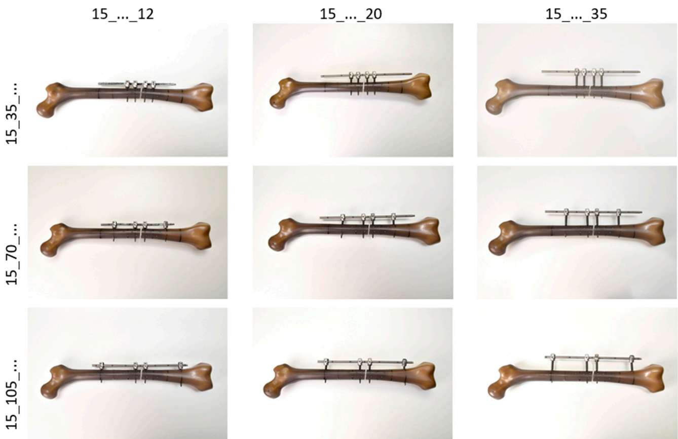
Figure 1. Overview of all variations of the pin2 and rod distances; the column-line labelling indicates the corresponding field in the 3 \times 3 test matrix according to the following syntax: Pin1(distance)_Pin2(distance)_Rod(distance).
