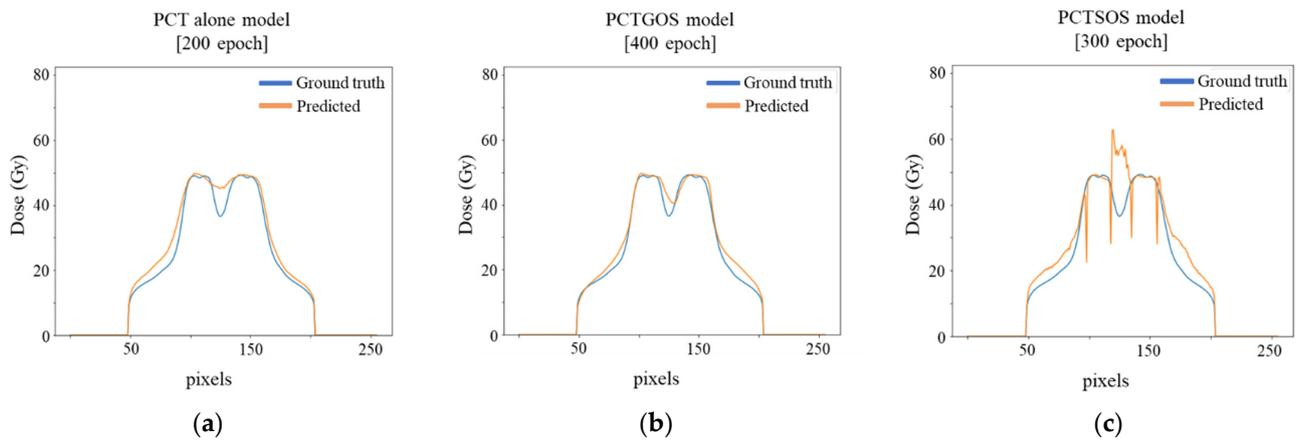
**Figure 4.** Dose profile comparison between ground truth (blue line) and predicted (orange line) dose distribution for 3 models: (a) PCT alone model; (b) PCTGOS model; and (c) PCTSOS model.
