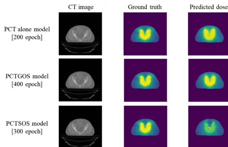
**Figure 3.** The input CT image, ground truth dose distribution, and predicted dose distribution results of the PCT alone model, PCTGOS model, and PCTSOS model.
