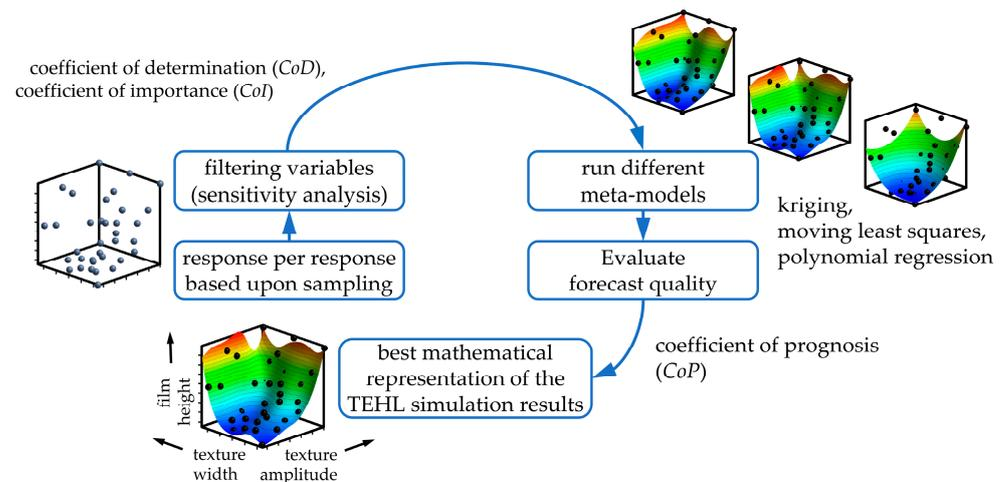
**Figure 6.** Framework of the metamodel of optimal prognosis to predict the tribological behavior of micro-textured EHL contacts utilized in [33].
