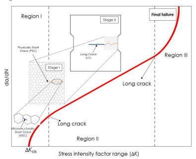
Figure 3. Schematic description of conventional fatigue crack growth behavior [13].
