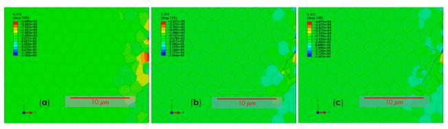
**Figure 12.** Damage initiation in the microstructural model of SAE 52100 martensitic hardened steel without voids in steps 1 (a), 10 (b), and 36 (c).
