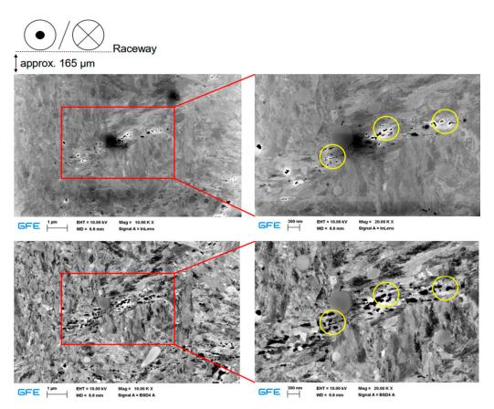
**Figure 6.** SE (**up**) and BSE (**down**) images of the microstructure in the depth of 165  $\mu$ m below the raceway. The porosities within the microstructure are signified by the yellow circles.
