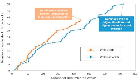
Figure 14. Comparison of the cycle accumulation for microstructures with and without voids.
