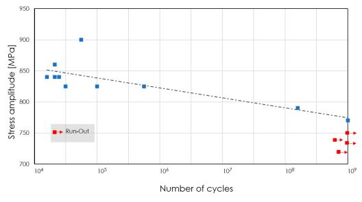
Figure 7. Experimental S-N diagram of SAE 52100 martensitic hardened steel [15].
