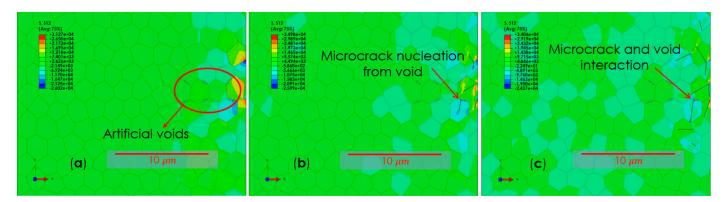
**Figure 13.** Damage initiation in the microstructural model of SAE 52100 martensitic hardened steel with voids in steps 1 (a), 10 (b), and 38 (c).
