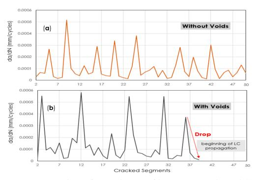
**Figure 11.** Comparison between fatigue crack initiation of the microstructures without voids (a) and with voids (b).
