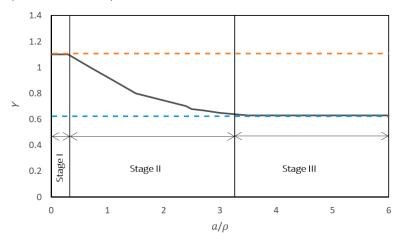
**Figure 2.** Geometry factor (*Y*) vs.  $a/\rho$  showing the three stages of crack growth from a spherical pore [12].
