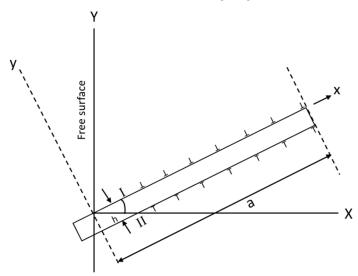
**Figure 8.** Schematic of a slip band as a combination of two parallel layers of dislocations colliding with a free surface at a specific angle.
