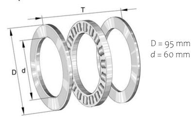
Figure 4. Axial cylindrical roller bearing (type 81212; Schaeffler).
