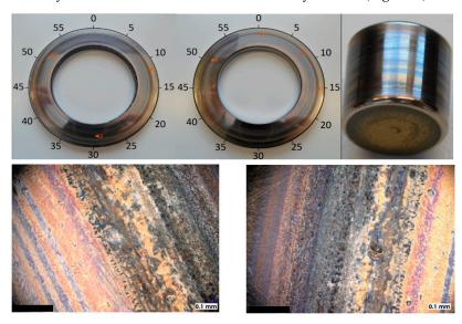
Figure 5. Alterations of the washers' surfaces from a damaged specimen.
