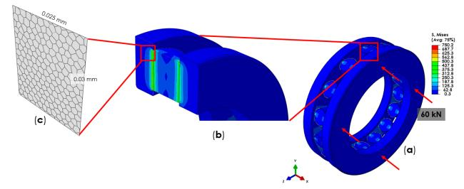
**Figure 9.** (a) Macro-model or global model of the bearing and the loading condition. (b) Cross-section of the macro-model in the contact area between the cylinders and the rings. (c) Micro-model developed in the area with the highest stress concentration.
