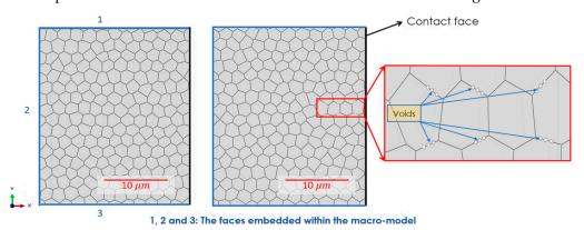
**Figure 10.** Microstructural models of SAE 52100 martensitic hardened steel, without pores (**left**) and with pores (**right**).
