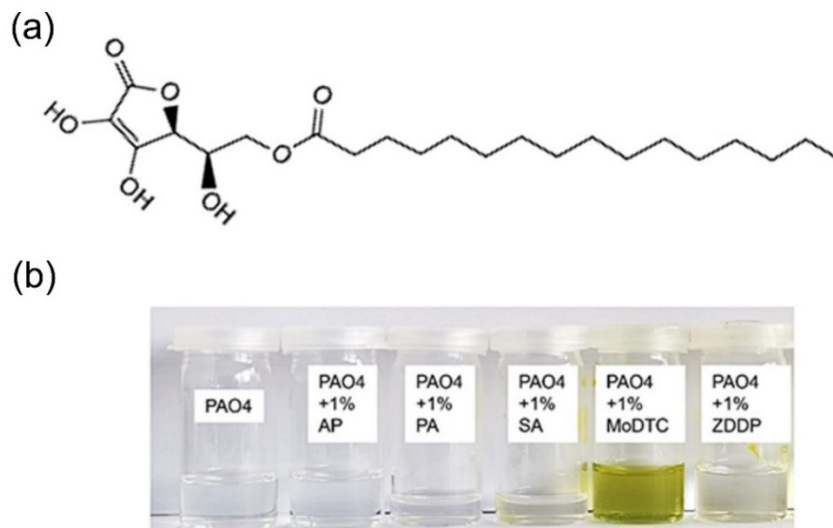
Figure 1. (a) Molecular structure of AP. (b) Optical pictures of mixtures of PAO4 with one wt% of each additive at 150 °C.
