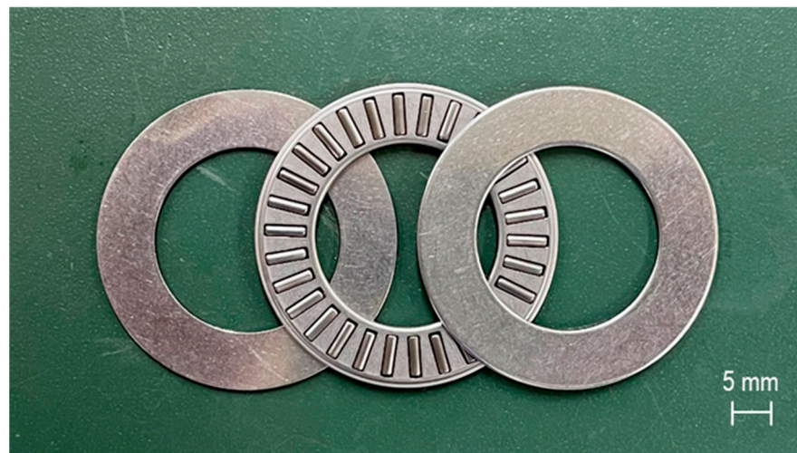
Figure 4. Photograph of a thrust needle roller bearing (FNTA2542) and the upper and lower races.
