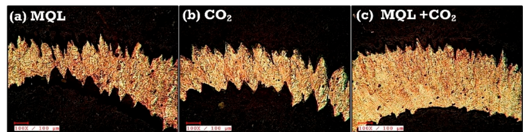
Figure 7. Chip morphology; V_c = 44 m/min, f = 0.04 mm/rev, and a_p = 0.43 mm.
