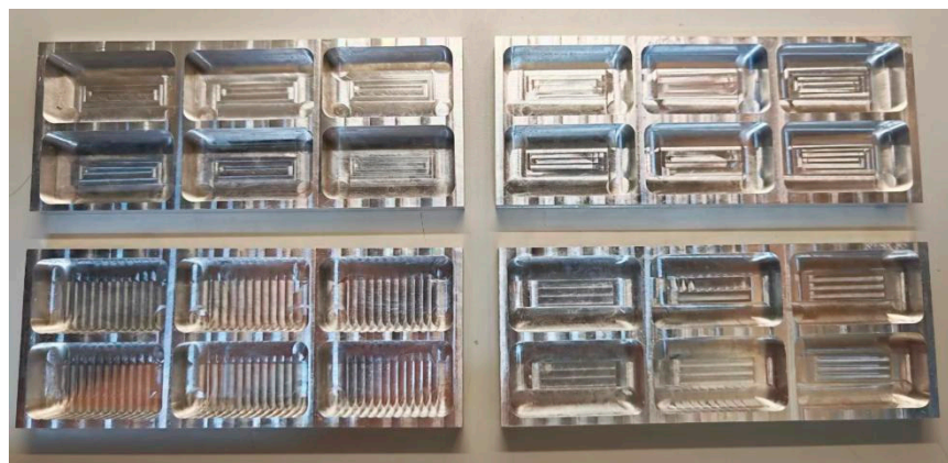
Figure 11. Structural components machined with different tool paths.
