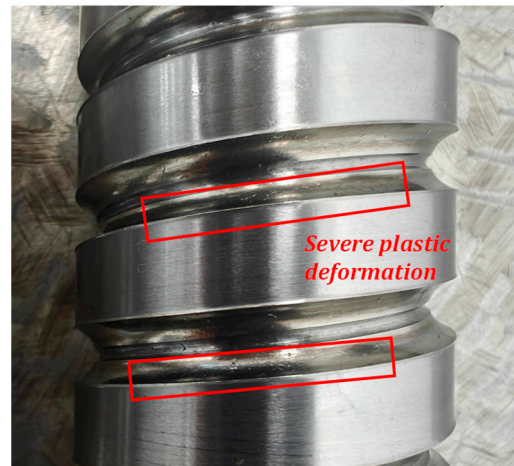
Figure 9. Plastic deformation of the 4016 specification screw raceway.
