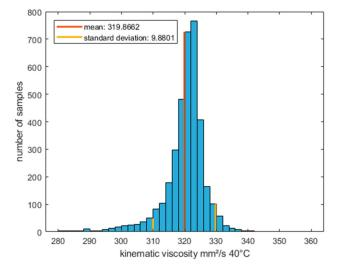
Figure 10. Distribution of the kinematic viscosity at 40 °C of PAO III.
