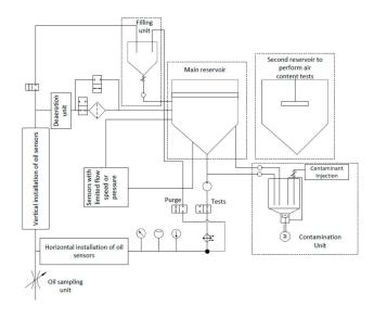
Figure 1. Layout of the oil sensor test bench at Fraunhofer IWES.
