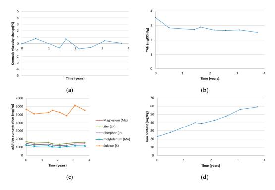
**Figure 6.** Sampling results of PAO II during the period of analysis. (**a**) Changes in the kinematic viscosity; (**b**) TAN; (**c**) additive content measured by the ICP method; (**d**) iron content measured by the ICP method.
