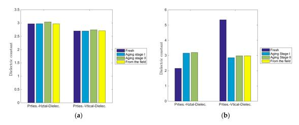
**Figure 2.** Measured dielectric constant of (**a**) mineral oil and (**b**) PAG oil during the stepped profile described in Section 3.2.2.
