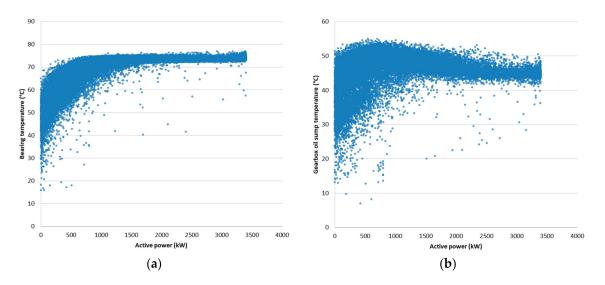
**Figure 7.** Gearbox temperature power functions during the first oil sampling interval of approx. six months. (a) Bearing temperature as a function of the active power ( $P_{act} > 0$ ); (b) gearbox oil sump temperature as a function of the active power ( $P_{act} > 0$ ).
