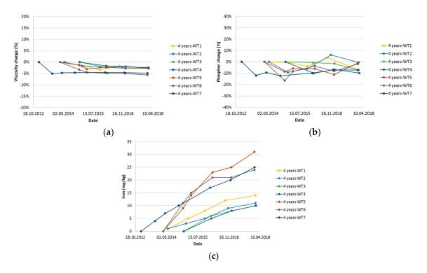
**Figure 8.** Trend analysis for the four-year turbine group with PAO I. (a) Changes in the kinematic viscosity; (b) changes in the phosphorus content measured by the ICP method; (c) iron content measured by the ICP method.
