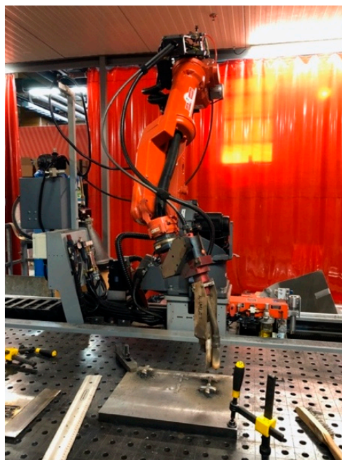
Figure 8. Welding robot as the main element of wire arc additive manufacturing (WAAM) printing.
