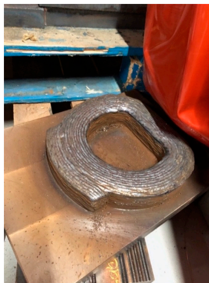
Figure 10. Crane hook during the 3D printing process.
