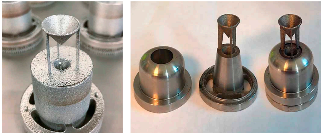
Figure 19. Nozzle manufactured by Wärtsilä [56].
