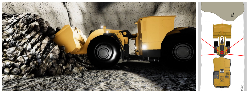
Figure 1. Image from a simulation of the LHD scooping muck from a pile. The right image shows a top view in which the positions of the lidar (five rays) and camera are indicated.
