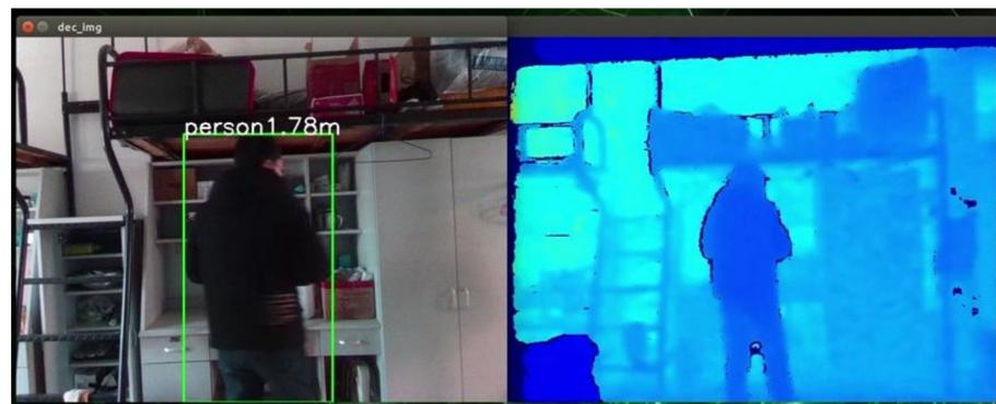
**Figure 10.** The real-time performance test for object detection on the NVIDIA Jetson NX embedded platform. The YZNet-YOLOV5-tiny system can simultaneously capture the target category with the distance provided by the depth image from the D435i camera. The complete video is available at: [https://www.bilibili.com/video/BV1G44y1J76B?share\\_source=copy\\_web](https://www.bilibili.com/video/BV1G44y1J76B?share_source=copy_web) (19 December 2021).
