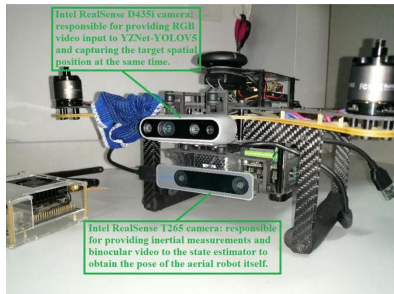
**Figure 1.** The aerial robot equipped with the RPEOD system.
