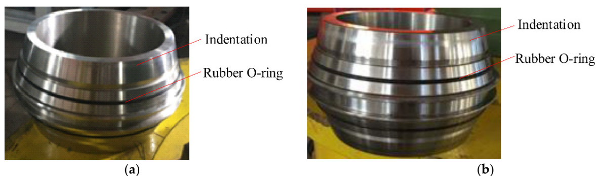
Figure 13. The state of the composite LSG after the test. (a) After the hydro-steady internal pressure test; (b) after the temperature cycle test.
