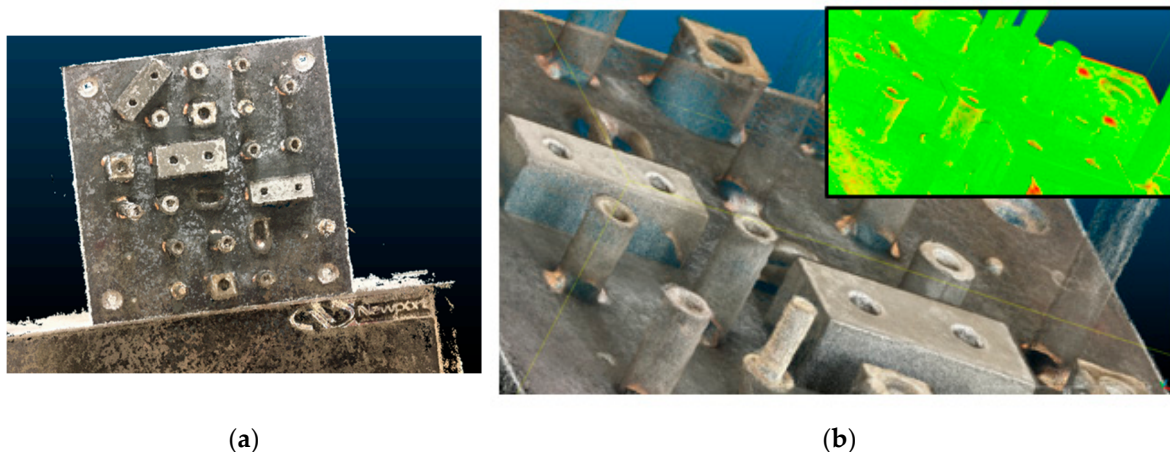
Figure 6. (a) Dense point cloud, (b) Close-up of the point cloud with distance map in the insert.
