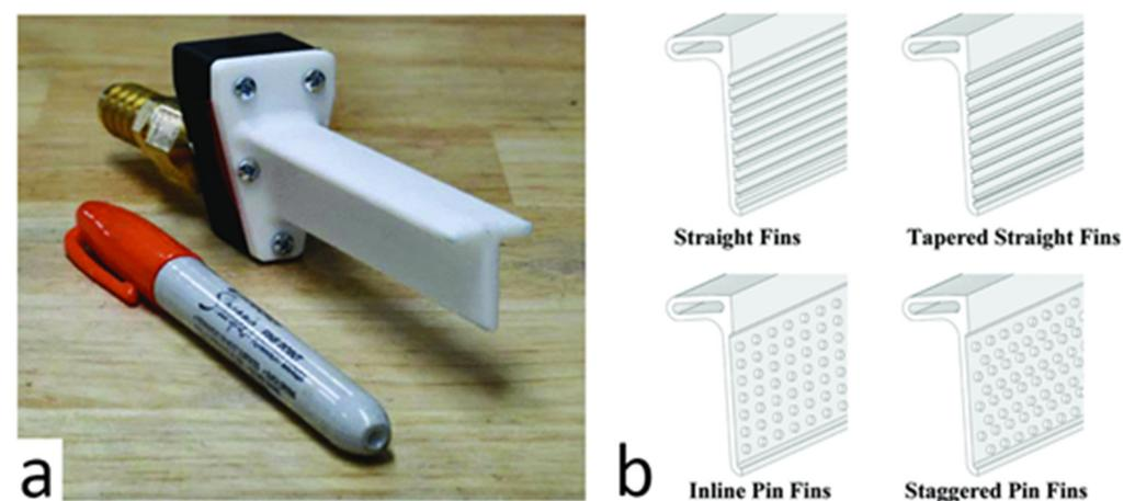
**Figure 15.** Additively manufactured ceramic heat exchanger for cooling the windings (a) and the different types of internal micro-features tested (b) Reprinted with permission from Ref. [43]. Copyright 2019 Elsevier.
