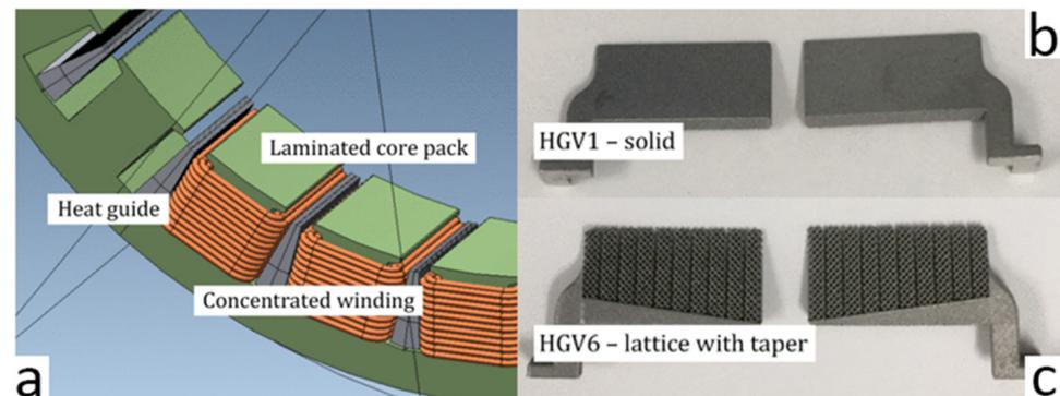
**Figure 14.** Additively manufactured heat guides places between the windings (a), a heat guide with a solid structure (b) and a heat guide utilizing a taper and a lattice structure to reduce eddy current losses (c) Reprinted with permission from Ref. [92]. Copyright 2020 Elsevier.
