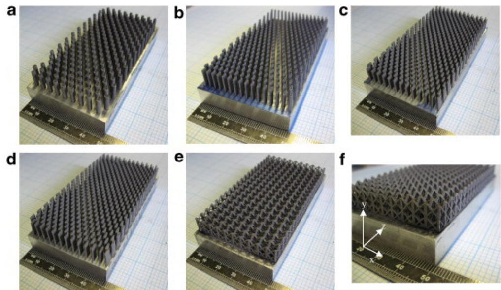
**Figure 8.** Additively manufactured pin fin heat sinks with different geometries: cylindrical pin (a), rectangular fin (b), rectangular fins with rounded corners (c), staggered elliptical array (d) and a lattice structure (e,f) Reprinted with permission from Ref. [69]. Copyright 2009 Elsevier.
