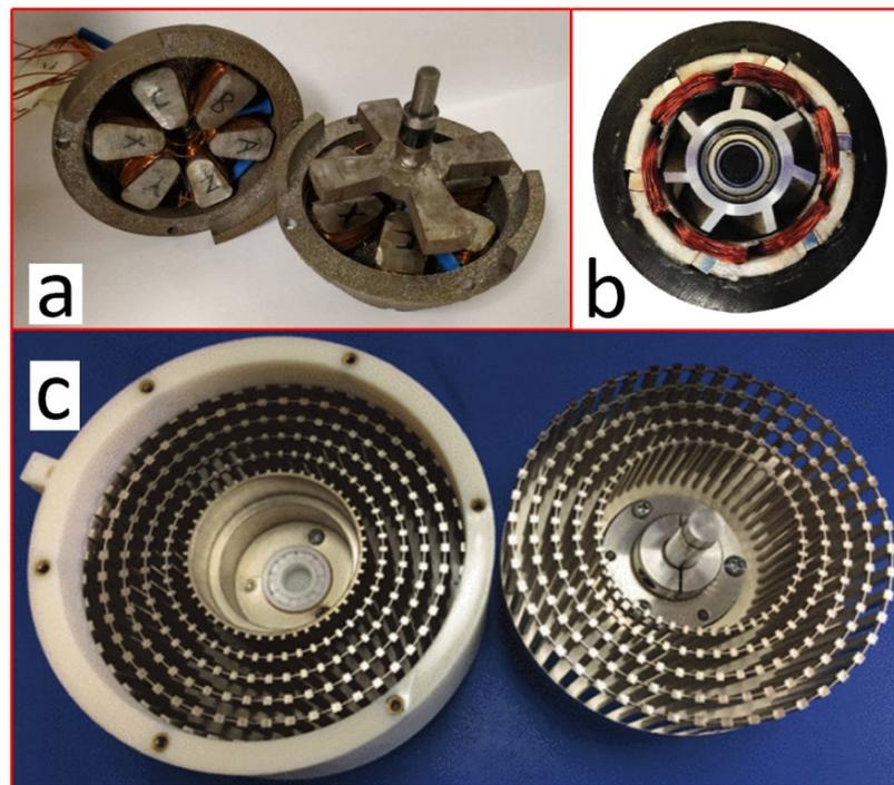
**Figure 4.** Additively manufactured electrical machines: (a) axial flux motor [47], (b) integrated fan motor reprinted with permission from Ref. [48]. Copyright 2021 Elsevier, (c) electrostatic motor [49].
