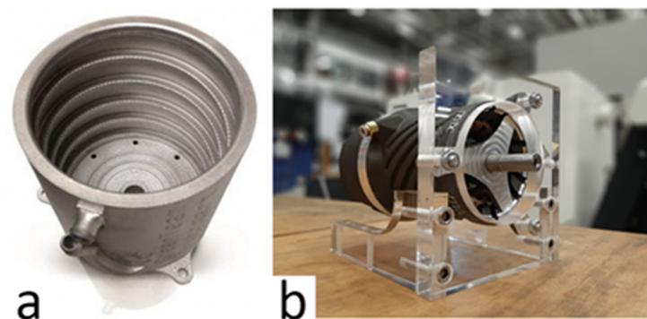
**Figure 11.** Additively manufactured cooling jackets (a) [74] and (b) [75].
