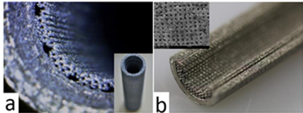
**Figure 13.** Additively manufactured heat pipes with an internal wick structure (a) Reprinted with permission from Ref. [84]. Copyright 2013 Elsevier and (b) Reprinted with permission from Ref. [88]. Copyright 2013 Elsevier.
