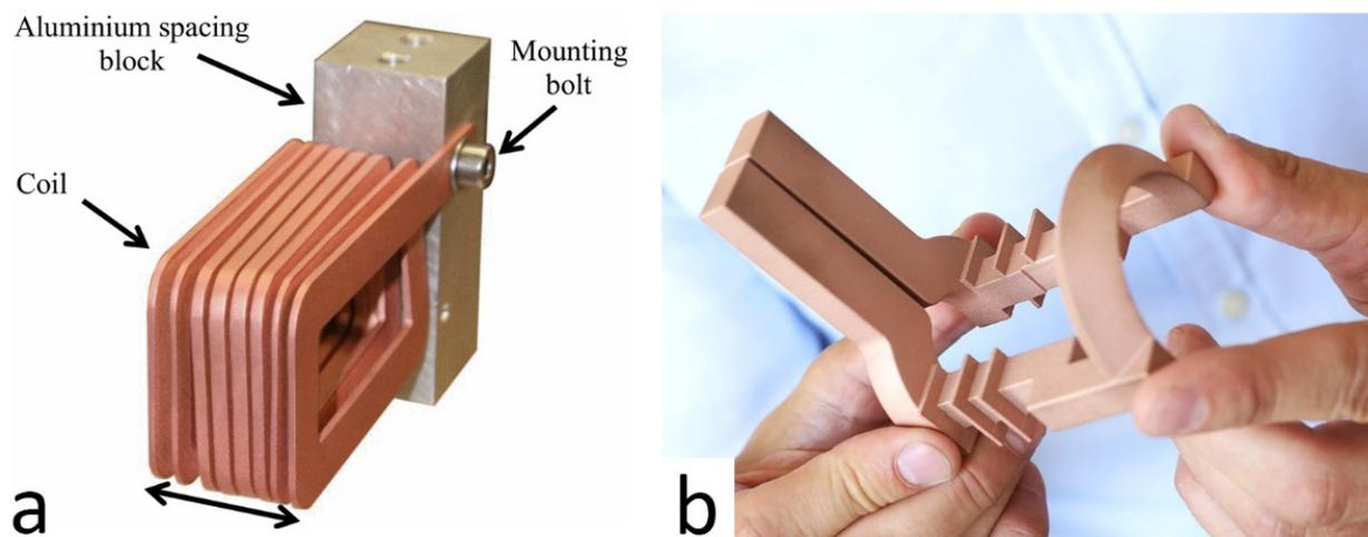
**Figure 3.** Additively manufactured (a) copper alloy windings [27] and (b) an induction heater with integrated water cooling [28].
