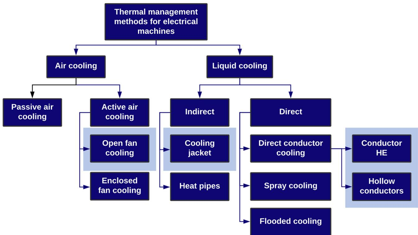
**Figure 5.** Various cooling methods for electrical machines. The light blue shading indicates that an additively manufactured solution for an electrical machine exists in the literature.
