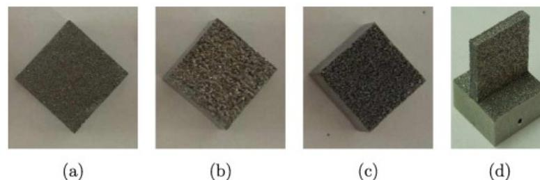
**Figure 10.** Aluminum alloy samples manufactured using DMLS with different average surface roughness: 16  $\mu\text{m}$  (a), 24  $\mu\text{m}$  (b), 43  $\mu\text{m}$  (c), 22  $\mu\text{m}$  (d) [72].
