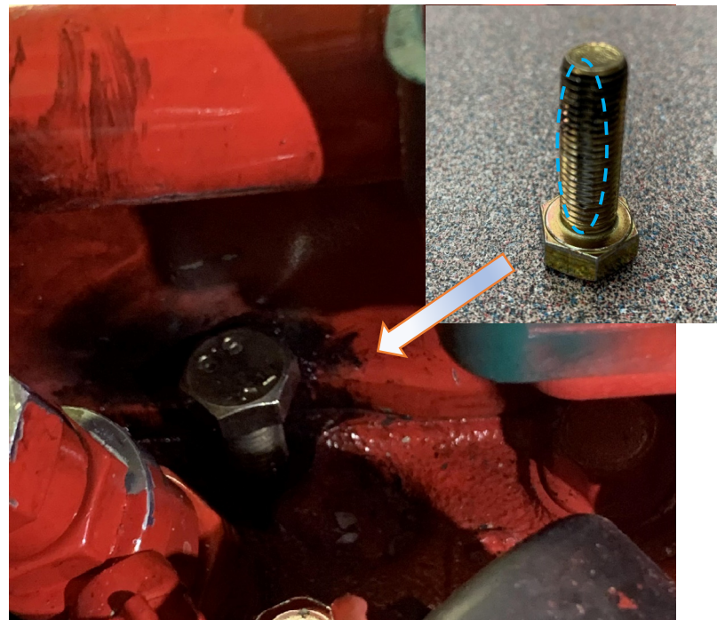
Figure 13. Cylinder leakage simulation.
