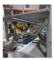
**Figure 17.** Part manufactured after the demolding. Filling and feeding systems are also shown in this image at Tecnalia's facilities (**left**). Inner Skeleton features (**right**).
