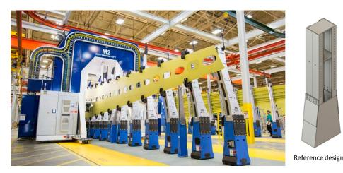
**Figure 2.** The wing skin panels for Boeing's first 737 MAX airplane are loaded on fixtures into an automated assembly machine in the company's plant in Renton, Wash., on 2 June 2015 (source: [33]) [left]. The simplified reference design of the assembly column based on the fixtures used in assembly lines [right].
