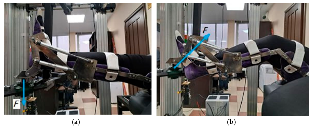
Figure 20. Test compression of elastic elements with simultaneous excess load along: (a) X-axis, (b) simultaneously along the X and Y, when a movement causes a simultaneous excess of load on both axes, compression of all pairs of elastic elements occurs.
