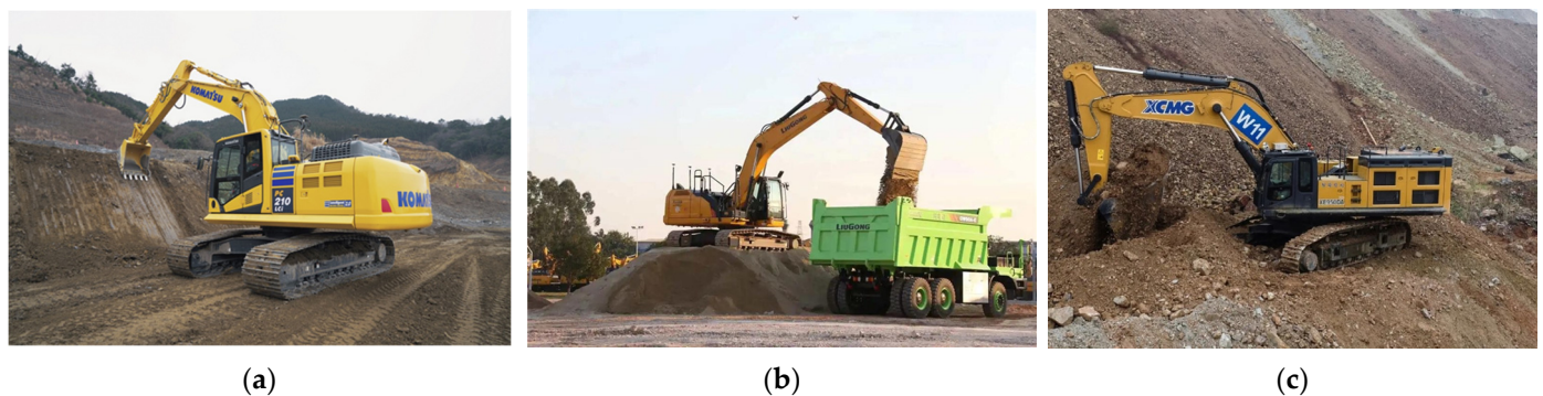
Figure 8. Various models of unmanned excavators: (a) Komatsu PC210LCi-11; (b) LIUGONG 922F; (c) XCMG XE950DA.
