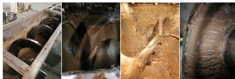
Figure 19. Negative pressure spiral separation dewatering device has a good solid–liquid separation effect.
