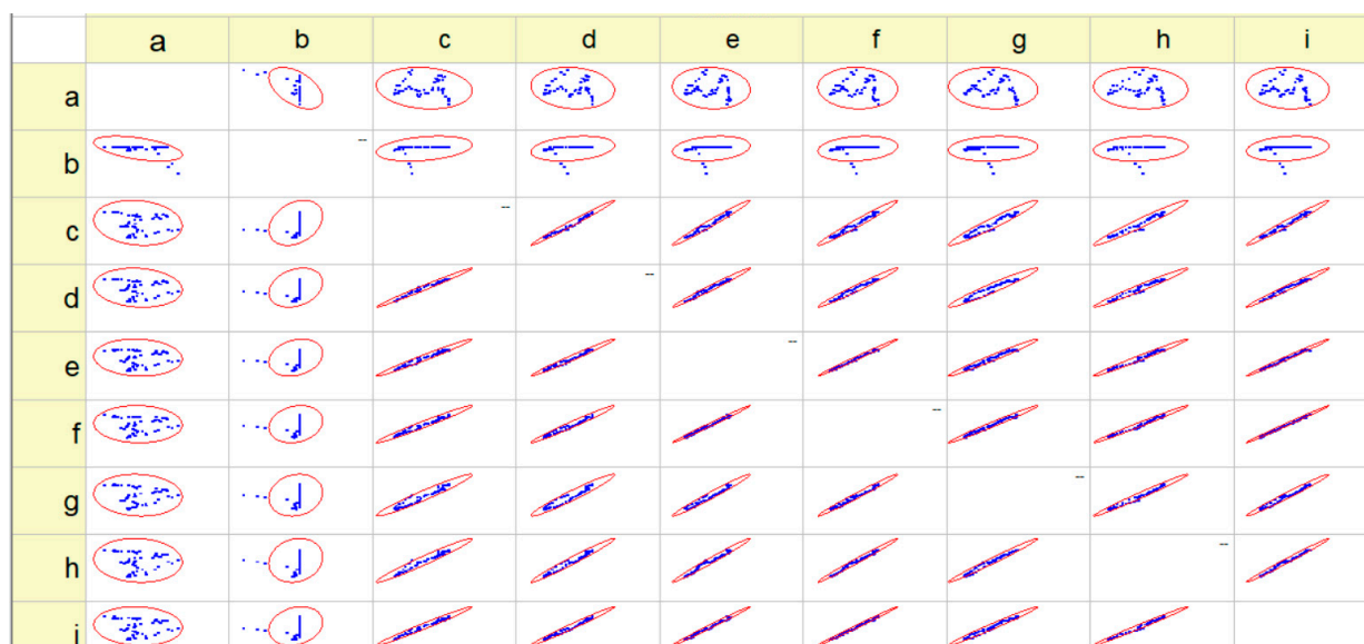
Figure 7. The correlation matrix is constructed from the calculated incoming and outgoing numerical particle concentrations of different particle sizes, giving the removal efficiency of the electrostatic precipitator for the different cases of system operation, a—background level of PM in the gas stream, b—electrostatic precipitator activation without feeding, c–i—electrostatic precipitator activation with the use of the different particle flux from the generator of aerosol.
