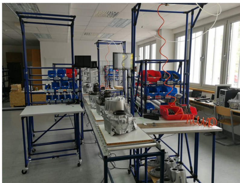
Figure 15. Gearbox assembly line in LF environment.
