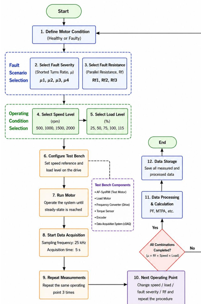
Figure 5. Experimental Data Acquisition and Signal Processing Flowchart.
