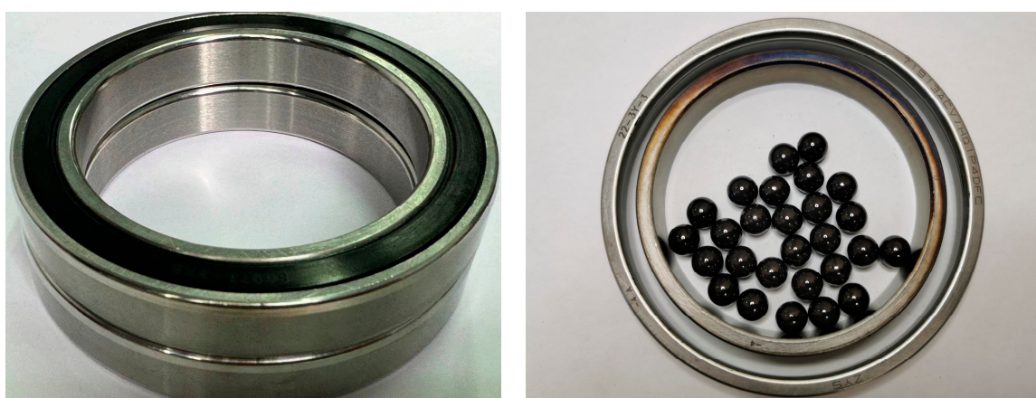
Figure 10. Auxiliary bearing used in the experiment.
