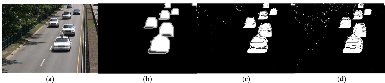
Figure 5. Qualitative results of CD net 2014 highway frame 1626. From left: (a) original frame, (b) ground truth, (c) Codebook algorithm and (d) GMM algorithm.
