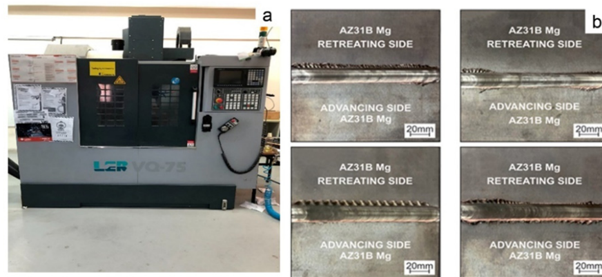
Figure 3. Experiment setup, illustration of typical weld bead surface appearance (a) universal milling machine (LER VQ75) used in FSW experiment, (b) weld surface under different process conditions [23].
