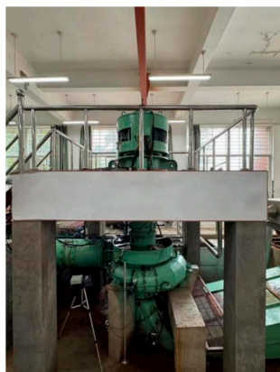
Figure 5. Francis turbine model test rig.
