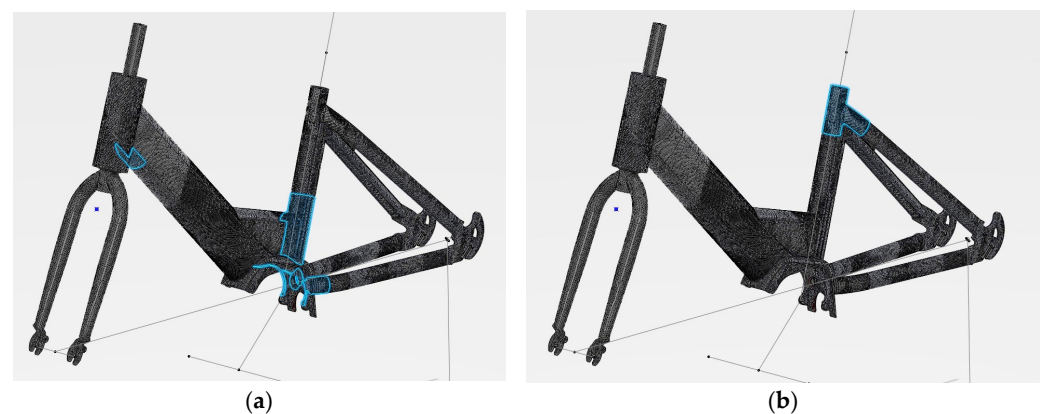
Figure 18. (a) Refinement areas with 1.75 mm mesh size on the Urban; (b) Refinement areas with 1.25 mm mesh size on the Urban.
