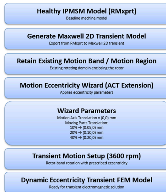
Figure 2. Workflow of dynamic eccentricity in ANSYS Maxwell, from the healthy model to the transient dynamic-eccentricity finite-element model.
