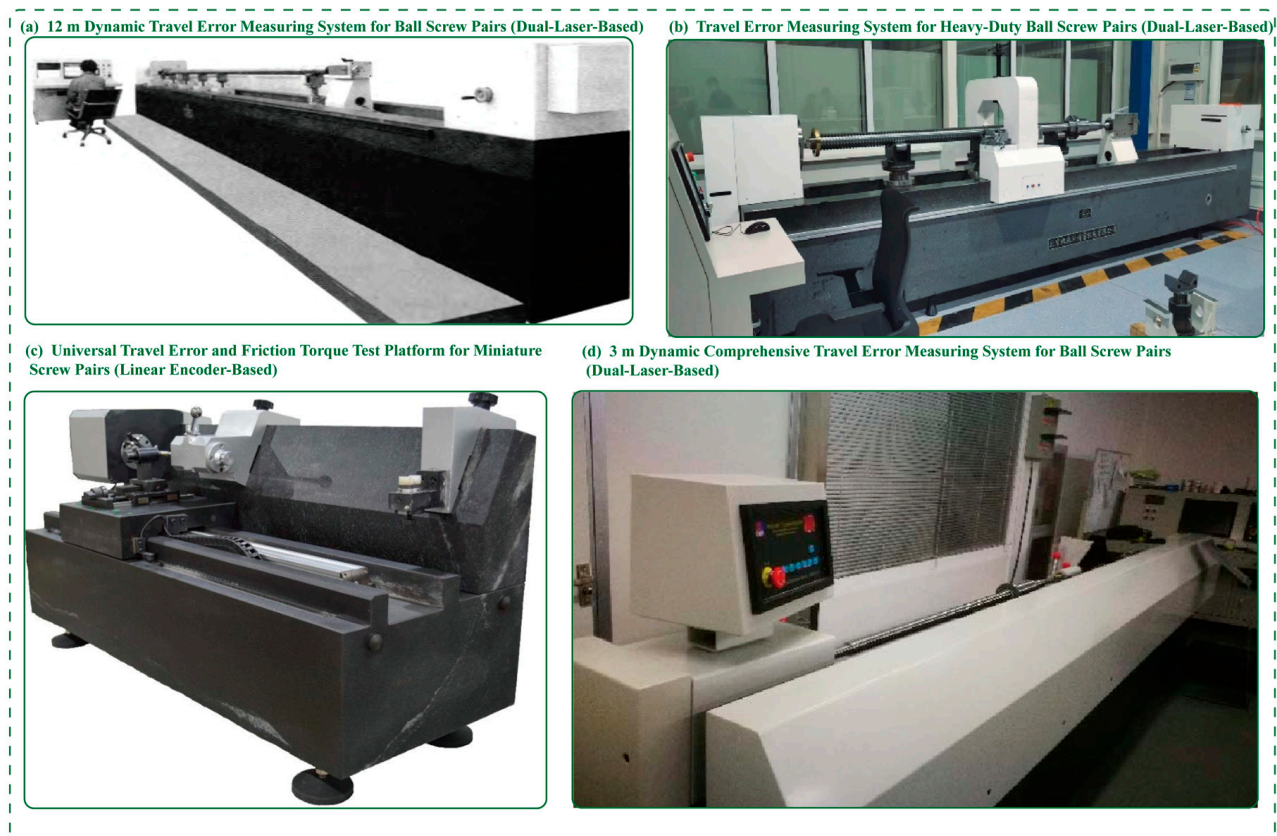
Figure 12. Photographs of representative measuring instruments [85,93,94]. (a) A 12 m dynamic travel error measuring system for ball screw pairs. (b) Travel error measuring system for heavy-duty ball screw pairs; (c) universal travel error and friction torque test platform for miniature screw pairs; (d) 10 m dynamic comprehensive travel error measuring system for ball screw pairs.
