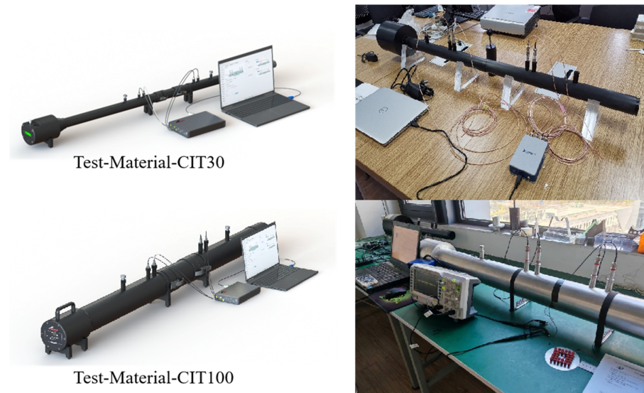
Figure 4. Test equipment: CIT30/100 impedance tube.
