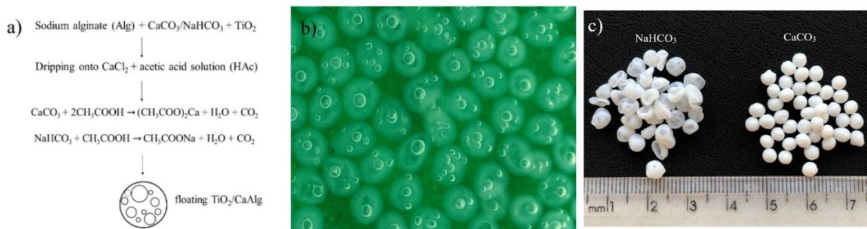
**Figure 6.** (a) Scheme from ionotropic gelation and CO<sub>2</sub> generation from both gas forming agents (CaCO<sub>3</sub> and NaHCO<sub>3</sub>), (b) bubbles held within the gel beads with CaCO<sub>3</sub> in its formulation, and (c) floating TiO<sub>2</sub>/CaAlg beads with 1:1 ratio of NaHCO<sub>3</sub>/alginate and 1:1 ratio of CaCO<sub>3</sub>/alginate [33].
