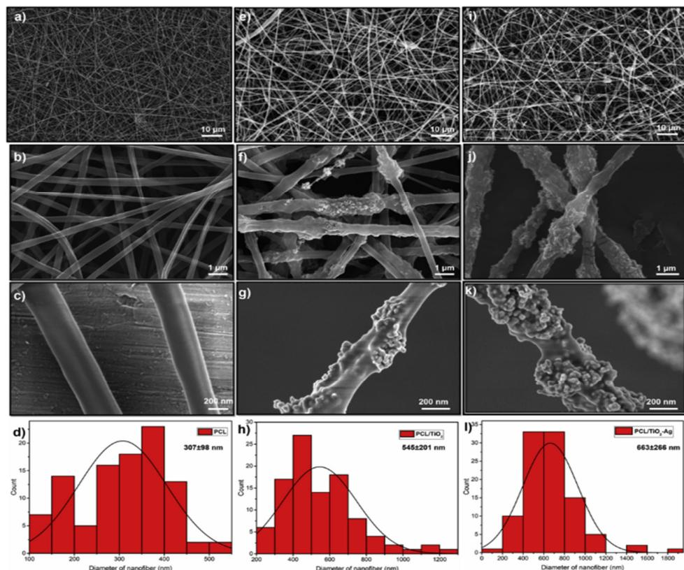
**Figure 11.** SEM images of (a–c) PCL, (e–g) PCL/TiO<sub>2</sub>, (i–k) PCL/TiO<sub>2</sub>-Ag NFs. Histogram presented the diameter distribution of (d) PCL, (h) PCL/TiO<sub>2</sub>, (l) PCL/TiO<sub>2</sub>-Ag NFs. Reprinted with permission of [46].
