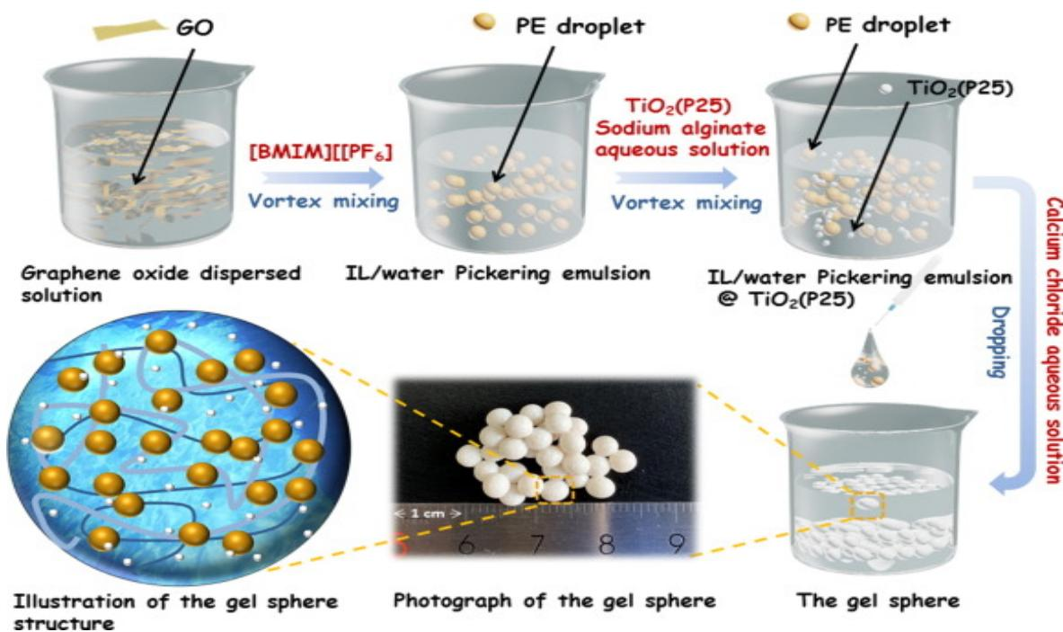
**Figure 7.** Schematic of the preparation process of the gel sphere [34].
