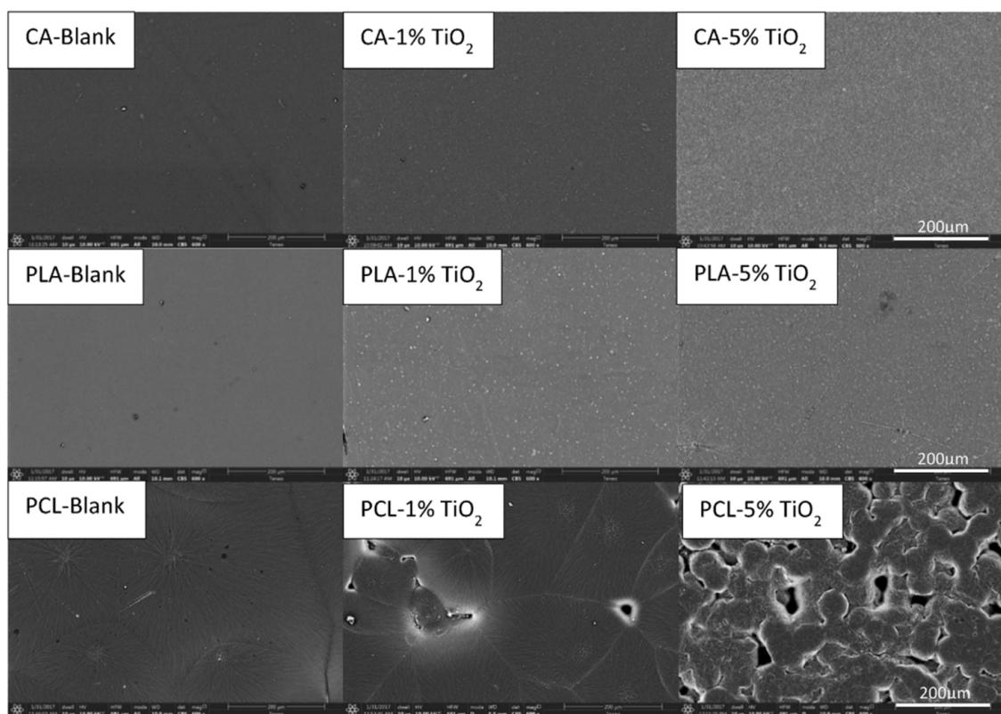
**Figure 9.** SEM images of  $\text{TiO}_2$  NPs embedded PLA, PCL and CA polymeric films. Reprinted from Reference [3].
