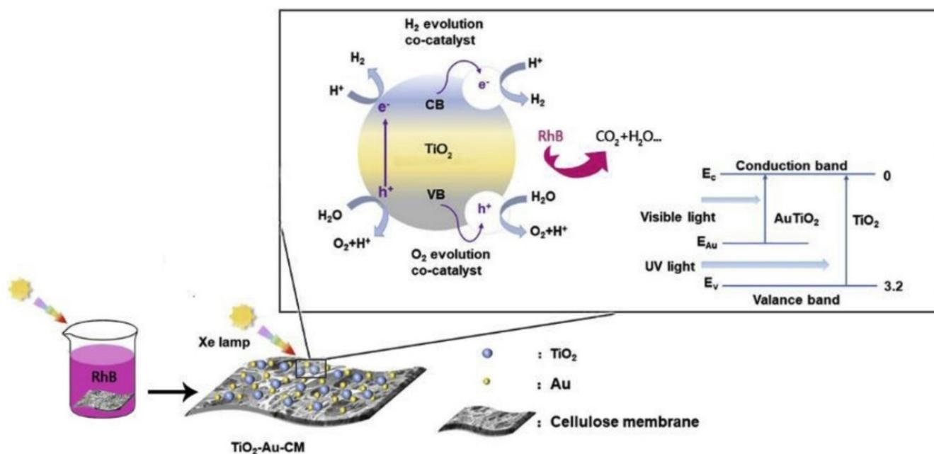
**Figure 3.** Schematic image for the mechanism of photoinduced charge carrier transfers in  $\text{TiO}_2\text{-Au}$  cellulose membranes under solar irradiation. Reprinted with permission of Reference [26].
