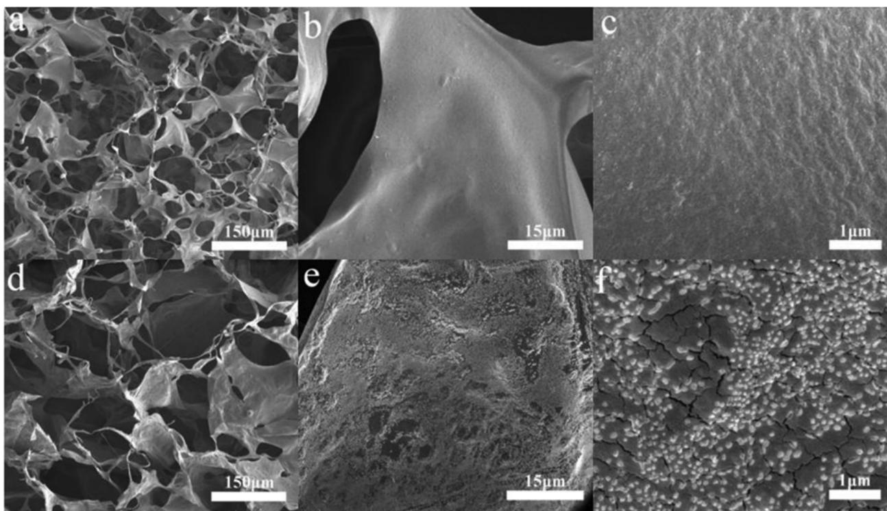
**Figure 8.** SEM images of the as-prepared SA aerogel (**a–c**) and SAT aerogel (**d–f**) with different magnifications. Reprinted from Reference [35].
