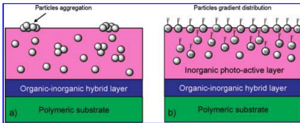
**Figure 10.** Schematic illustration of the multilayer functional coating on PLA substrate with (a)  $\text{TiO}_2$  nanoparticles without surface fluorination, (b) surface fluorinated  $\text{TiO}_2$  nanoparticles [6].
