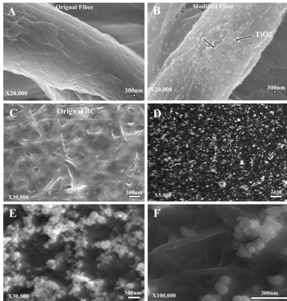
**Figure 4.** SEM images of unmodified fibers of cellulose filter paper (**A**) and after formation of CP/TiO<sub>2</sub> film (**B**), FEG/SEM image of original BC membrane (**C**) and after formation of CP/TiO<sub>2</sub> film on BC in low (**D**) and high magnification (**E,F**). Reprinted with permission of [30].
