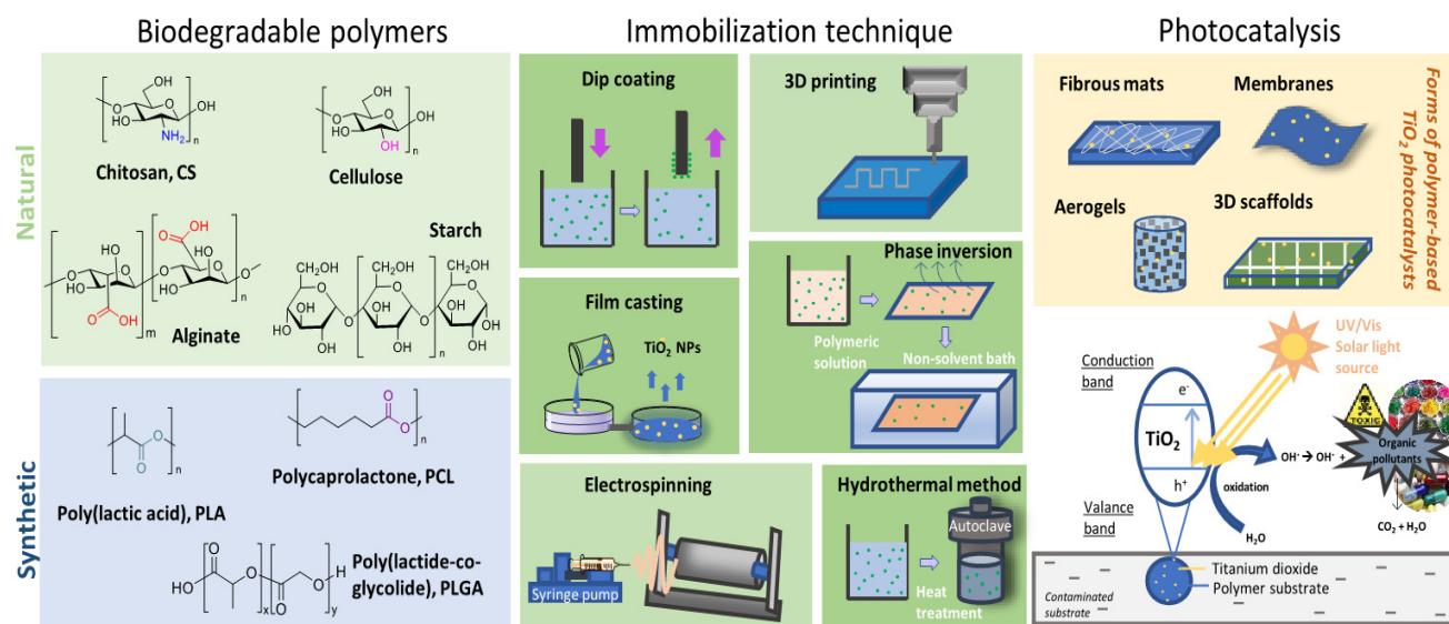
**Figure 1.** A brief illustration of the main synthetic routes fabricated for the immobilization of  $\text{TiO}_2$  nanoparticles onto biodegradable polymeric substrates for the photocatalytic degradation of organic pollutants.
