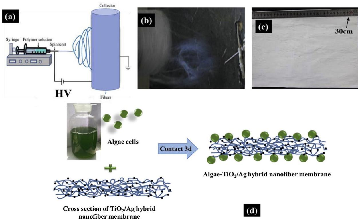
**Figure 2.** (a) Schematic illustration of electrospinning system, (b) nanofibers generation by single needle electrospinning, (c) demonstration of large-scale nanofibers mat and (d) scheme modeling the preparation of algae decorated TiO<sub>2</sub>/Ag hybrid nanofiber membrane. Reprinted with permission from [24].
