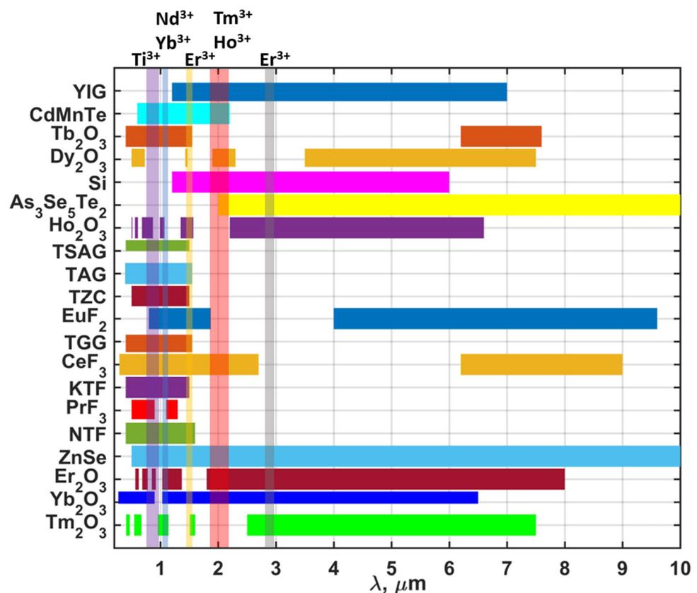
**Figure 1.** Transmission spectra of magneto-optical materials. Arranged in descending order of the Verdet constant value from top to bottom. Translucent vertical stripes indicate the characteristic spectral regions in which lasers based on the specified above ion can generate radiation.
